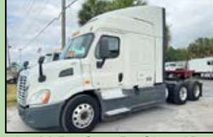
'18 Freightliner Cascadia - CA 1135LP, mid roof, DD13, 12.8 L, 450 hp, A/T DT 12-DA - 1550, HD 12 spd. direct drive, 12k front, 40k rear, 2.4/1 ratio 557k mi. $37,500.
