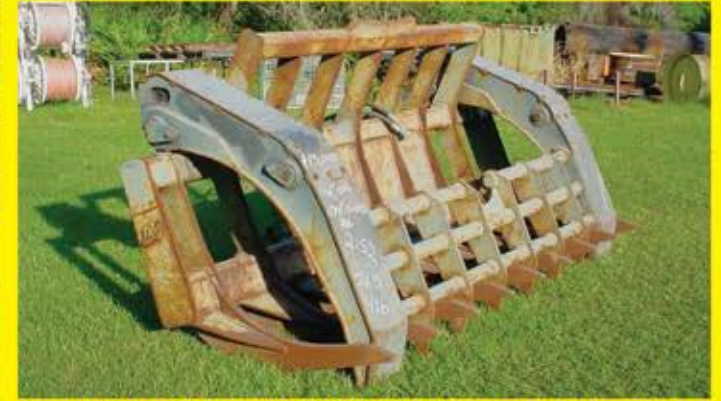
Grapple Rake - JRB coupler, 116"W, 104" at tines, excellent condition. $15,000.
