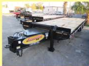
'24 Econoline DP2027DA Dual Tandem 20 ton 27' Equipment Trailer Dual 2 speed jacks, chain storage, Oak decking, LED lights, (2) 20,000# axles, air brakes, 215-75R17.5 tires, 48,000#GVW. $28,995+12%FET.
