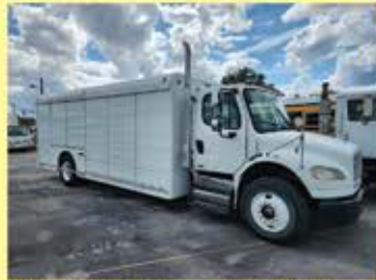
14565A - '09 Freightliner M2106 - 12 Bay Beverage Body , ISC Cummins 260HP, 6 speed, A/C, 253K miles, cruise, air brakes, 295-75R22.5 tires, 33,000# GVW. $19,900.
