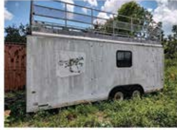
Media Event Trailer - Roof over upper deck, completely electric outfitted, tandem axle, heavy duty, forward compartment for Genset, etc.
