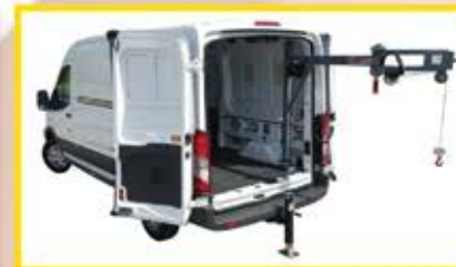
Venturo Van Crane - 1,000 lb cap., 64 ft. lbs. crane rating, 6' telescopic extended boom reach, 4'6" stowed boom length, 220 lbs., winch 12V DC, 1.3 hp motor, 25.5 fpm. $5,500 installed.
