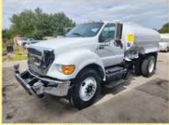
Q26335 - '15 Ford F750XL Valew 2,000 gal. Truck - 6.7L Cummins, 6 spd, A/C, 10K mi, cruise, 5 cab controlled sprayers, 3" water transfer pump, air brakes, 11R22.5 tires, 25,999# GVW. $72,900.
