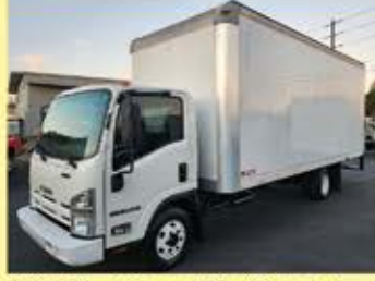
Q262339A - '14 Isuzu NPR - 20' van body , 6.0L V8 gas, auto, A/C, 124K miles, cruise, P/W, P/L, AM/FM CD radio, step bumper, LT215-85R16 tires, 12,000# GVW. $32,900.
