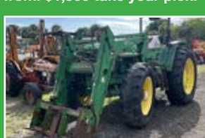
John Deere 6410 - 4x4, 4 cyl. turbo diesel, 640 loader, quick attach, lift arms, pto, 2 remotes. $15,000.
