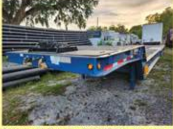
Q26319 - '17 Trail-King TKB0HT-533 - 53'x 102" tri-axle lowboy trailer , 40+ ton cap., hyd. beaver tail, hyd. winch, air-ride, alum. wheels, 235-75R17.5, lift tires, 255-70R22.5 tandem tires. $68,900.
