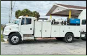
00 Freightliner FL 70 - Mercedes engine, 6 spd air brakes, 33k GVW, pto driven air compressor, Bobcat Miller 250 welder, auto crane body, 6k boom, 6006H 16' body, 22.5 alum. wheels, very-deep rubber, work ready, outriggers, Reese hitch. $43,500.
