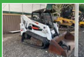
Bobcat T650 - 4 cyl., v3307 Kubota diesel, 2,802 lb. lift capacity, rubber tracks, OROPS. $29,500.
