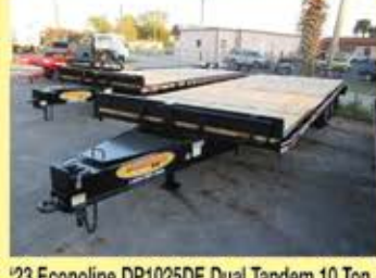
'23 Econoline DP1025DE Dual Tandem 10 Ton 25' Equipment Trailer - Chain storage , locking lid, (2) 10,000# axles, LED lights, electric brakes, 235-80R16 tires, 25,500# GVW. $13,295.
